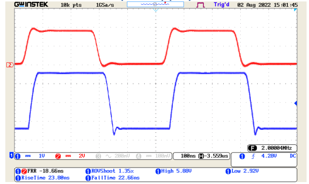
Output Overdriven Recovery, 3 V to 6 V, FAST_EN = 1 RS = 22 \Omega , CL = 50 pF, RL = 1 K \Omega (SELECT) (VO)
