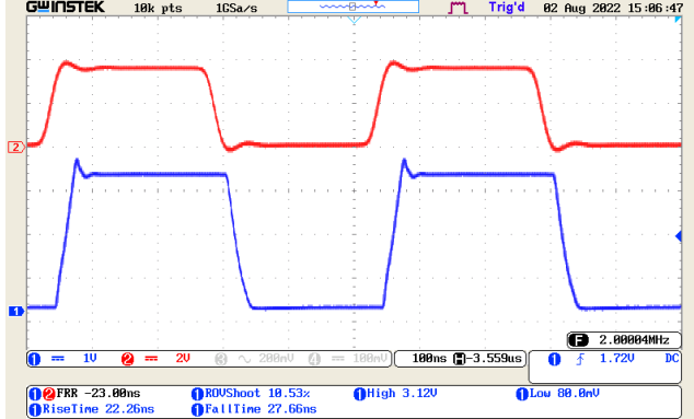
Output Overdriven Recovery, 0 V to 3 V, FAST_EN = 1 RS = 22 \Omega , CL = 50 pF, RL = 1 K \Omega (SELECT) (VO)
