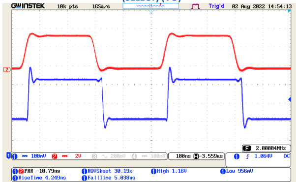
small signal 1 V to 1.2 V Step @ V_{DD\_ANA}=4.5 V, V_{DD\_DIG} = +3.3 V FAST_EN = 0 RS = 22 \Omega , CL = 50 pF, RL = 1 K \Omega (SELECT) (VO)
